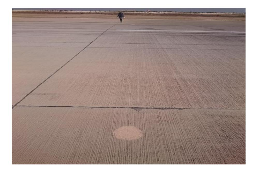
3- Macrotexture assessment using sand patch method as per ASTM procedure. A total of 200 sand patches have been implemented to cover the assessment requirements.
